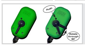
The Actuators **Art.3005-3006** and **Art.3007-3008** are equipped with a manual release, which allows manual opening or closing of the zone valve in the event of power failure.
