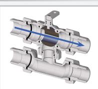
The figure shows the flow of fluid towards the supply manifold, when the valve is fully open.
