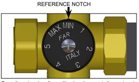
Once the mixer handle position has been set, the system is calibrated. The values indicated in the table above can vary ( $\pm 2^{\circ}$ C tolerance), depending on the characteristics of the system where the unit is installed. Final adjustment can be made by referring to the value indicated on the ball valve temperature gauge.
